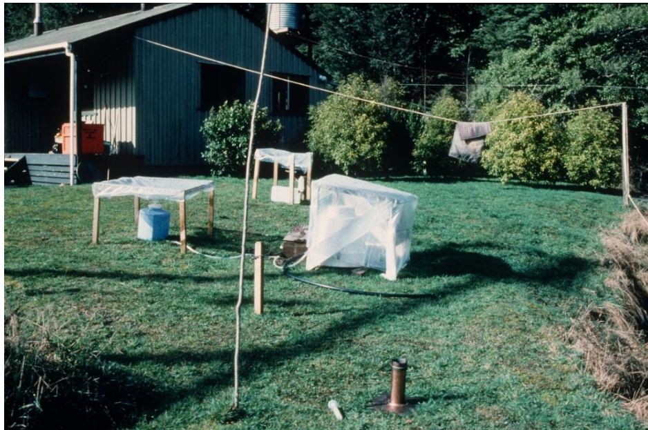
Figure 3. Rainfall samplers and corner of DOC hut at Maimai.
