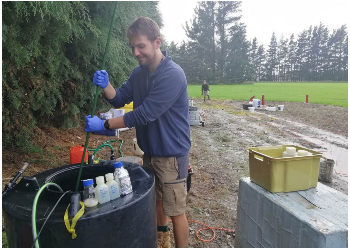
Figure 1. Andrew Pearson (ESR) preparing the injection mix for the bacterial and viral indicator tracer experiment to characterise the fate and transport characteristics of the site.
