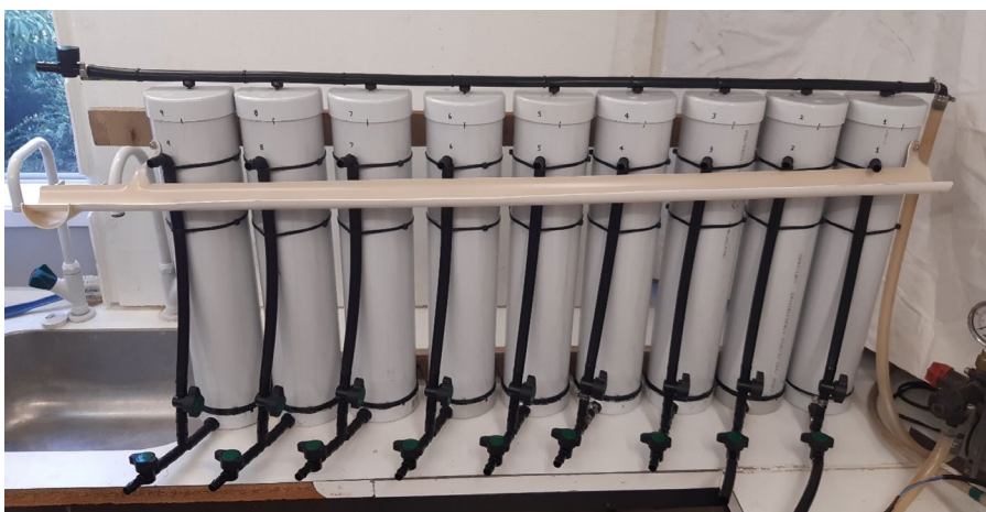
Figure 3. Lab-based bioreactor column experimental set-up. Each cylinder is filled with woodchips or a combination of woodchips and biochar with iron/manganese oxides.
