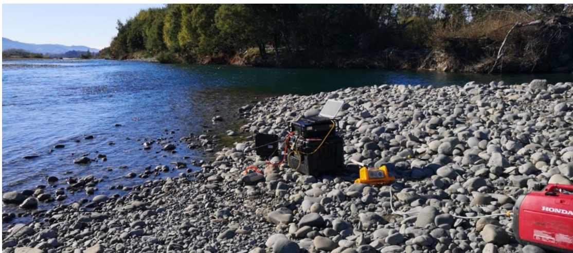
Figure 2. Measuring temperature variation across a pool in the Wairau River using distributed temperature sensing (DTS).
