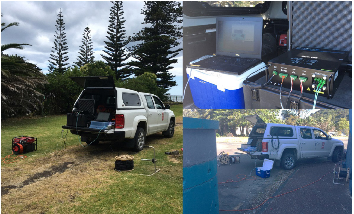
Figure 2: Deployment of FODTS method at Waiwera (January 2020) showing FODTS equipment in the back of a field vehicle during deployment and monitoring of borehole temperatures.
