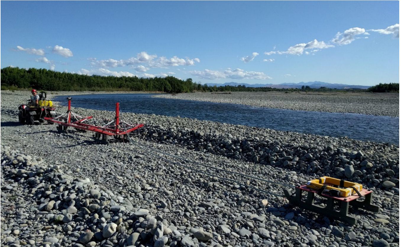
Figure 4: The Braided Rivers Programme uses a towed transient electromagnetic (tTEM) survey to gain information about the resistivity of materials forming the bed of the Wairau River.
