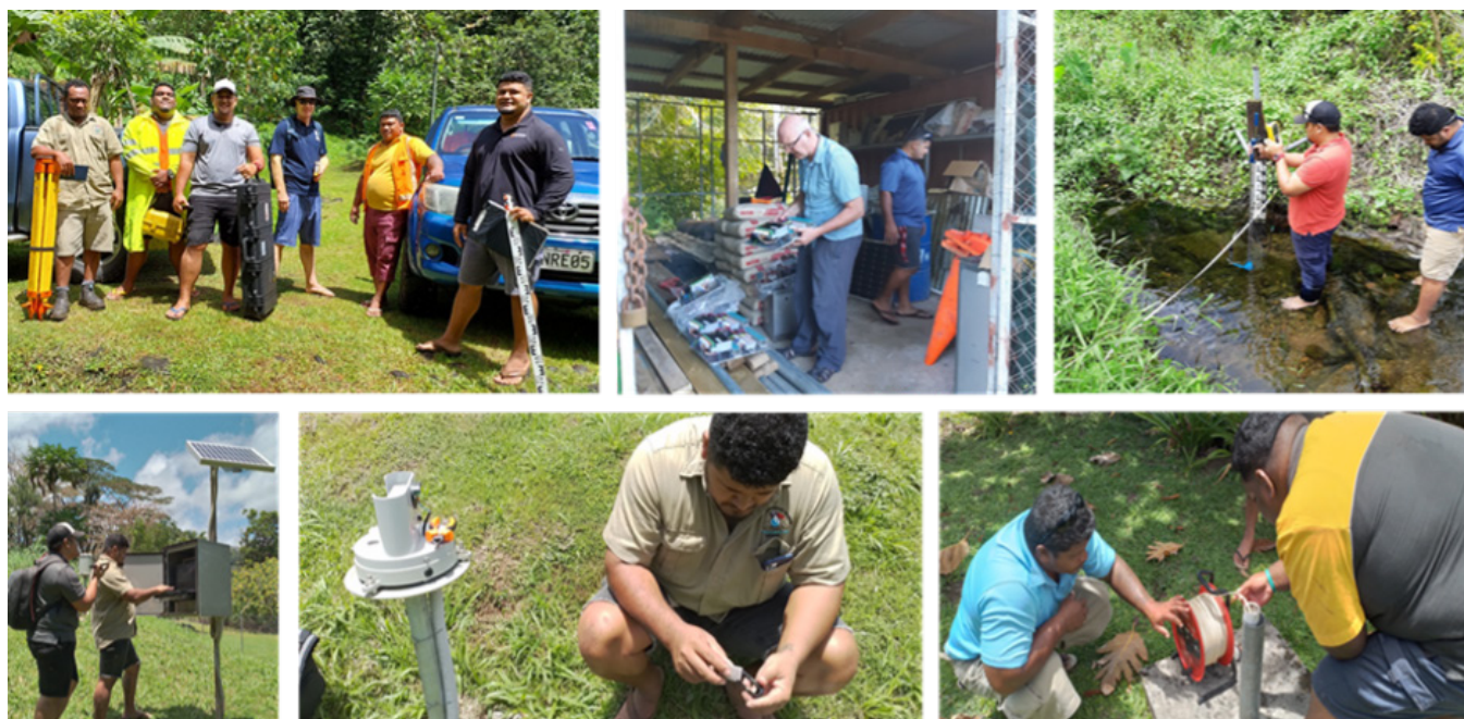
NIWA and Samoa WRD staff (top left); preparing data loggers (top middle); flow gauging (top right); data logger and telemetry maintenance (bottom left); maintaining rain gauge (bottom middle); and groundwater monitoring (bottom right). Photos: M. O'Driscoll, E. Baddock and S. Williams.
