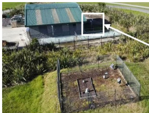
24 and 9 GHz profilers and tipping bucket rain gauges at Anawhata (left) and a 24GHz profiler operated adjacent to a rain gauge enclosure equipped with both tipping bucket and weighing rain gauges in Orewa (middle/right).
