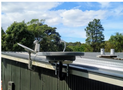
24 and 9 GHz profilers and tipping bucket rain gauges at Anawhata (left) and a 24GHz profiler operated adjacent to a rain gauge enclosure equipped with both tipping bucket and weighing rain gauges in Orewa (middle/right).
