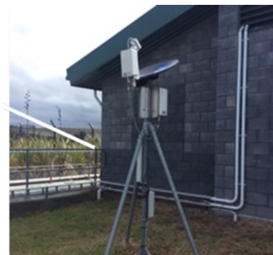
24 and 9 GHz profilers and tipping bucket rain gauges at Anawhata (left) and a 24GHz profiler operated adjacent to a rain gauge enclosure equipped with both tipping bucket and weighing rain gauges in Orewa (middle/right).
