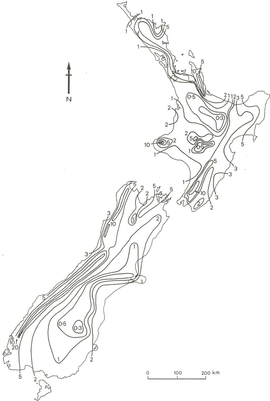
Figure 1.7. Distribution of mean annual flood peak ( \text{m}^3/\text{s}/\text{km}^2 ). Mean annual flood is divided by catchment area A^{0.8} . (from McKerchar and Pearson 1990)
