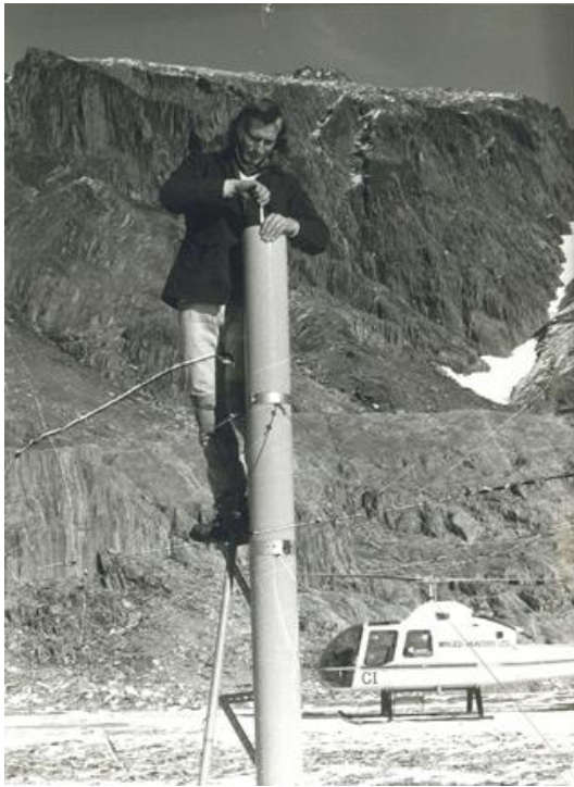
Figure 2 (left): Beaumont Basin raingauge, 14 June 1978. Graeme Horrell reading the rainfall total since the previous visit. Figure 3 (right): Cropp River at Waterfall raingauge. Hydrological Society Conference field trip on 20 November 2008. (Later, between 22–25 November, 991 mm rain was recorded.) From left: Bob McDavitt, Mathirimangalam Srinivasan (MS), Suzanne Poyck and Graeme Horrell.
