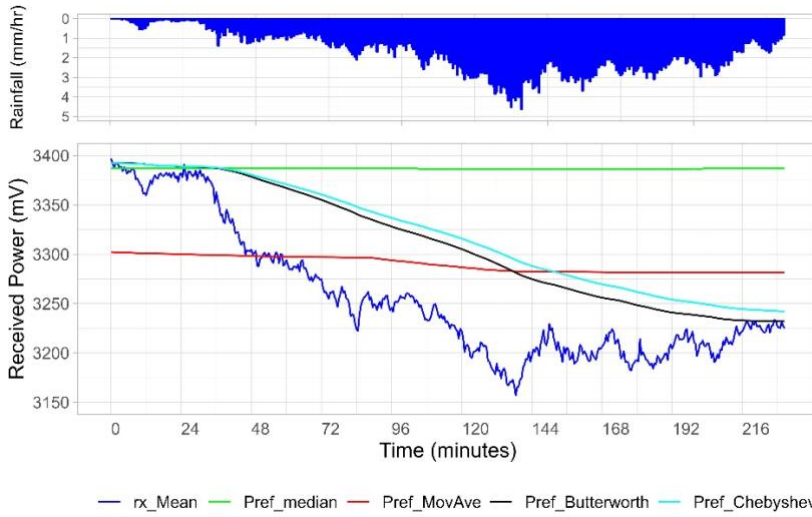
• Figure 1: Comparing the base power in filtering methods with the conventional median method
