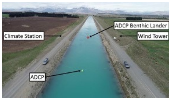
Figure 1: Field measurements of velocity profiles and wind in the Tekapo Canal, New Zealand.
