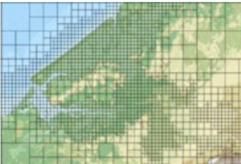
Figure 1. Refined block quadtree created by BG_FLOOD. The colour shading is the catchment topography where each pixel represents a model cell, the black lines represent the extent of a block of 16x16 model cells.
