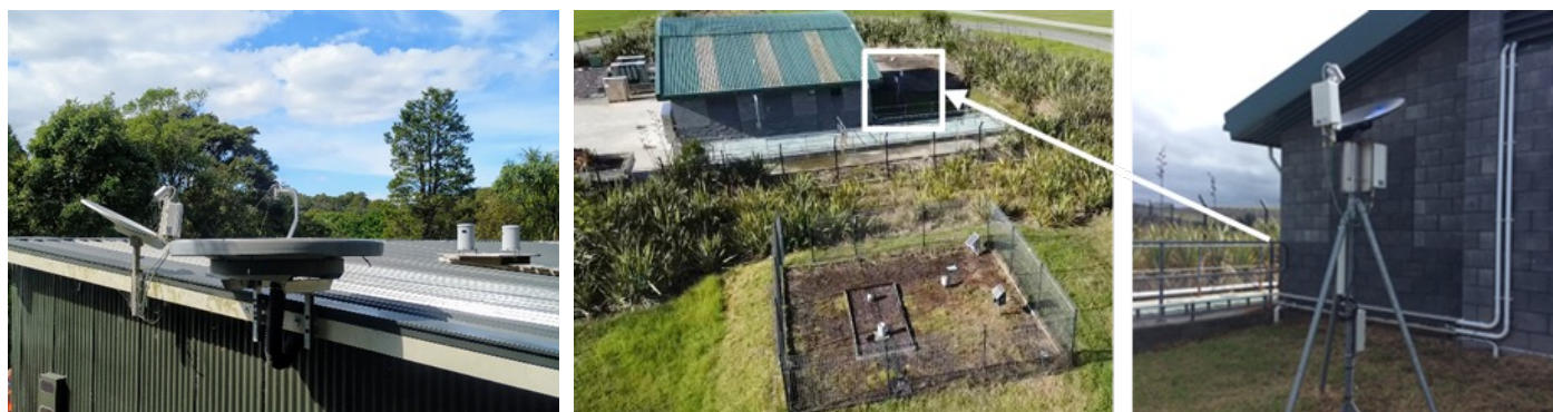
24 and 9 GHz profilers and tipping bucket rain gauges at Anawhata (left) and a 24GHz profiler operated adjacent to a rain gauge enclosure equipped with both tipping bucket and weighing rain gauges in Orewa (middle/right).
