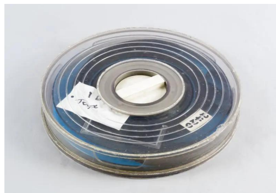
Figure 3 – A 2400 foot long magnetic tape
