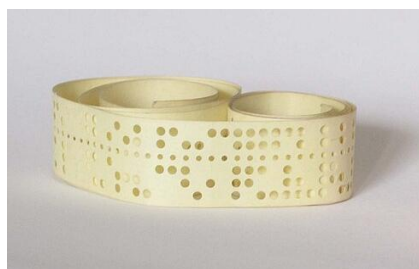
Figure 2. Five-hole wide punched paper tape
