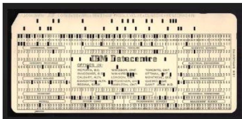
Figure 4 – An 80 column computer card
