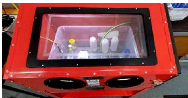
Figure 3: The anaerobic chamber constructed from a repurposed sand blasting cabinet
